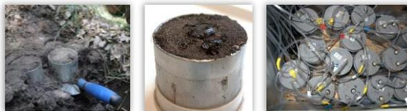
Fig. 1: Sampling of soil cores (left), 250 cm<sup>3</sup> soil core ready for analysis (middle) and vessels for soil cores inside the measuring unit for N<sub>2</sub>O, CH<sub>4</sub> and CO<sub>2</sub>
